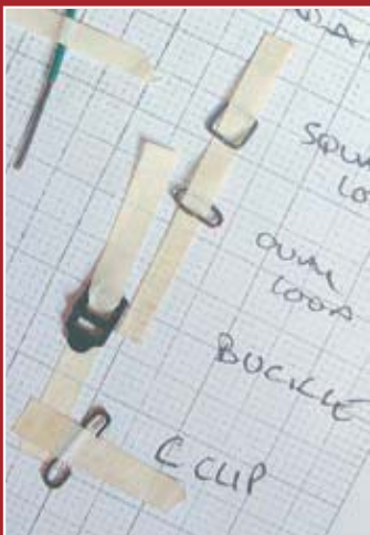
The prototype webbing was constructed using scratch built buckles
