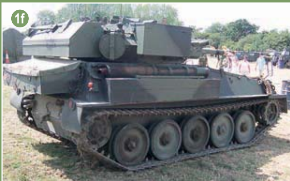
1f Track sag, note how the upper run of track is entirely unsupported
