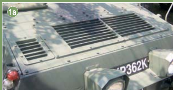
1a Bolted transmission cover (on a preserved Scorpion). Correct for Falklands Scorpion
