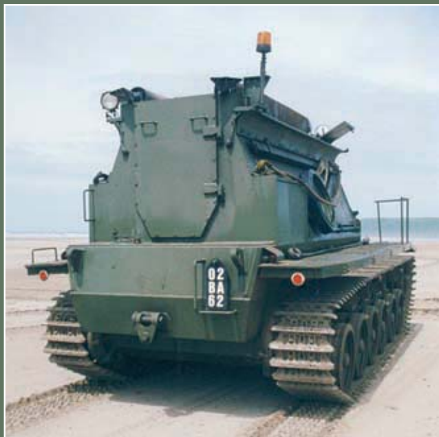
Nice rear three-quarter view of the Centurion BARV showing the layout of the rear hull. Shown clearly here is the large bolted access door for the engine compartment as is the curvature of the splash rails that run around the top of the superstructure, which prevents the sea entering the top of the vehicle.
