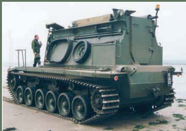
Overall rear three-quarter view, same BARV on Instow beach. The BARV is around 20 inches (50.5 cm) taller than a Mk3 Centurion gun tank, but can ford in depths up to 9½feet. A spare wheel half is carried either side of the superstructure and various other tools and pieces of equipment are stowed in brackets around the vehicle, making the BARV pretty much self-sufficient when operating in the field.
