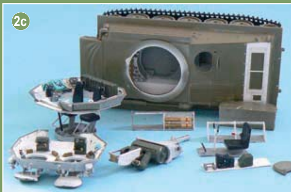
Interior constructed from scratch, painted and ready to be fitted into place. Note also view of scratch-built transmission cover
