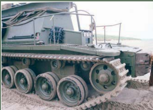
This BARV has the later style front idler wheel. Note how the front section of the 'catwalk' comes very close to the top of the tracks. The large wooden nudge block at the front is clearly shown. This was a later addition when it was found that vehicles or vessels being pushed could be damaged if being pushed at an angle.
