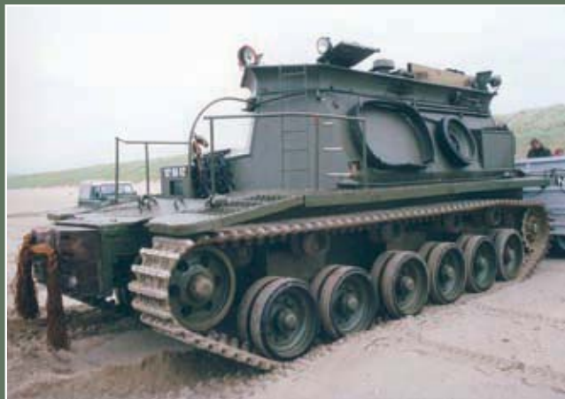
Centurion BARV on the beach at Instow in Devon, home of ATTURM (Amphibious Trials & Training Unit Royal Marines). These Centurions have now been pensioned off and replaced by the state-of-the-art Leopard-based Hippo. The grey vehicle behind the BARV is a wartime DUKW that was and I think still is being used by the Marines as a support vehicle!
