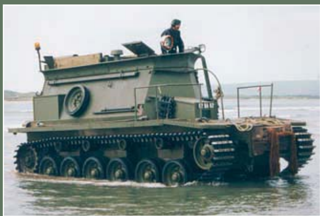
Overall rear three-quarter view, same BARV on Instow beach. The BARV is around 20 inches (50.5 cm) taller than a Mk3 Centurion gun tank, but can ford in depths up to 9½feet. A spare wheel half is carried either side of the superstructure and various other tools and pieces of equipment are stowed in brackets around the vehicle, making the BARV pretty much self-sufficient when operating in the field.
