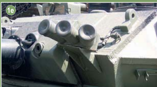
1e Three-barrelled smoke discharger, required for Falklands Scorpion
