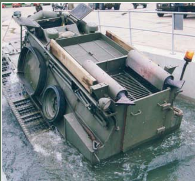
This is a very useful photo to refer to when constructing the mesh 'catwalks' down either side of the vehicle. The 'catwalks' are used to reduce buoyancy when the vehicle is wading in the water, allowing the water to come through the panels rather than push upwards against them if they were solid. You can also see the additional loops welded to the glacis plate that are used as attachment points for the ropes when towing. Note the white horizontal bars attached to the front section of the superstructure that indicate the depth of water.
