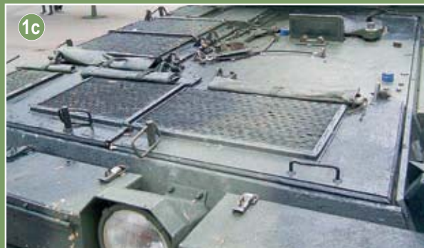
1c Hinged transmission cover (on Scimitar in service). Provided with kit
