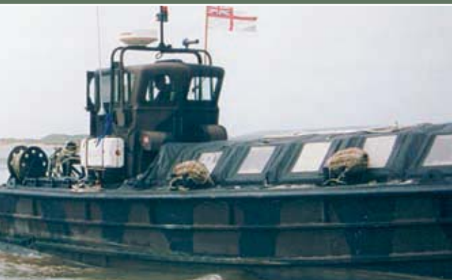
Right: As the BARV leaves the dip tank it gives a fine view of the roof top details. The two louvered vent sections, rear mounted exhausts and wooden blocks are clearly visible. The large rear door is only ever opened if the engine needs to be removed, other than that it remains bolted and sealed to the elements. The only way in and out of the BARV is through the front hatch.
