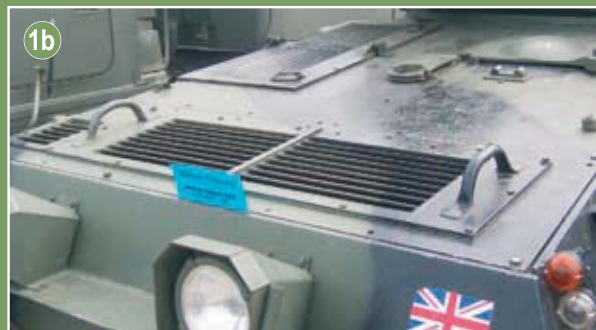
1b Bolted transmission cover with handles (on a preserved Scorpion)
