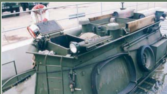
With the BARV in the dip tank we can see the details at the front end of the superstructure roof. Note the shape of the chimneys, the fire extinguishers and aerial mount between them, as well as the curved shrouds for the pipe leading to the exhaust within the louvered section at the rear.
