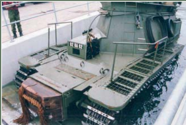
This is a very useful photo to refer to when constructing the mesh 'catwalks' down either side of the vehicle. The 'catwalks' are used to reduce buoyancy when the vehicle is wading in the water, allowing the water to come through the panels rather than push upwards against them if they were solid. You can also see the additional loops welded to the glacis plate that are used as attachment points for the ropes when towing. Note the white horizontal bars attached to the front section of the superstructure that indicate the depth of water.
